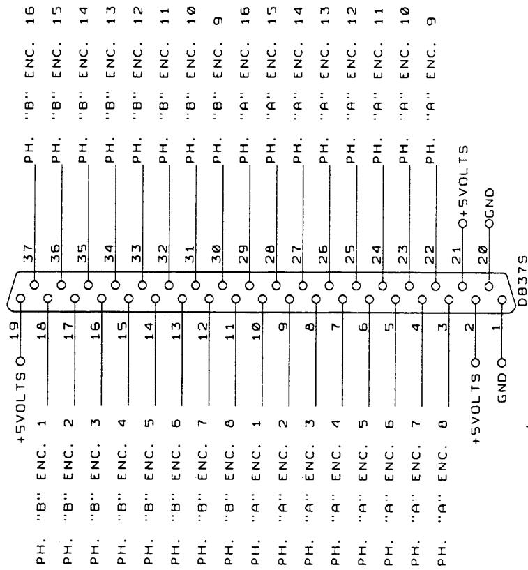
IT IS POSSIBLE TO HOOK UP ENCODERS WITHOUT THE BLACK BOX. THE ABOVE SCHEMATIC SHOWS THE ENCODER CONNECTIONS WHEN CONNECTOR "JP4" ON THE RTMC48 CARD IS BROUGHT OUT TO A MALE DB37P CONNECTOR AT THE BACK OF THE COMPUTER. IT IS ASSUMED THAT PIN ONE OF JP4 AND PIN ONE OF THE DB37 ARE CONNECTED TOGETHER VIA THE RED WIRE ON THE RIBBON CABLE.
